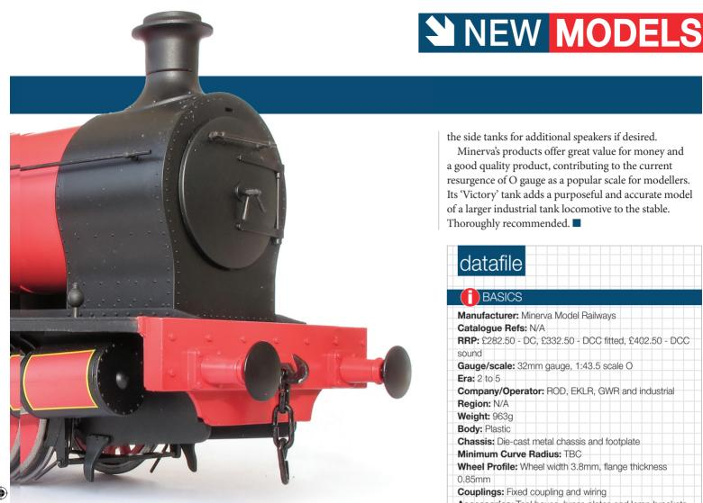
The model is a weighty 963g, giving smooth and quiet performance and a very respectable haulage capacity. Electrical pick-up is via all six wheels with a high-torque flywheel-equipped motor which drives the rear axle through a 40:1 gearbox giving slow, smooth running.
